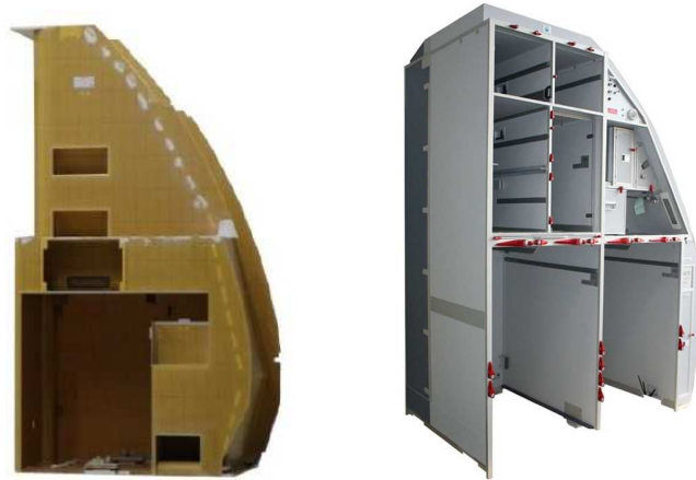
Figure 1.1.: Narrow body of a galley under construction by sandwich composite (left) and final product for both Airbus and Boeing narrow body platform (right), photos from [1].
