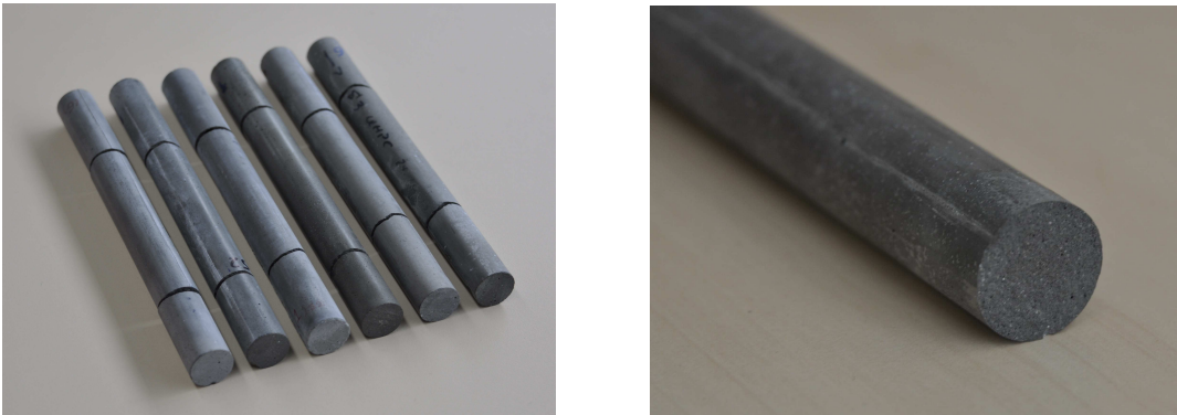
Figure 5.18.: UHPC specimens fractured in the spalling tests (left) and a typical fracture surface (right).
