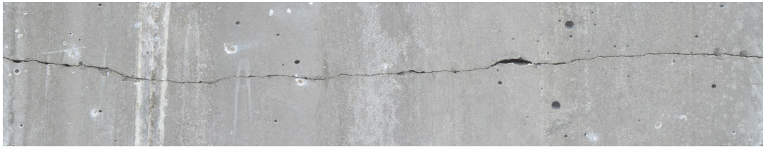
Figure 5.20.: Full circumferential contour of a cracked S_1 specimen composed of 33 single photographs.
