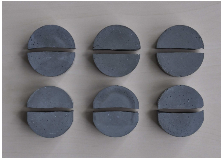
Figure 5.26.: Broken circular and flat end UHPC specimens.
