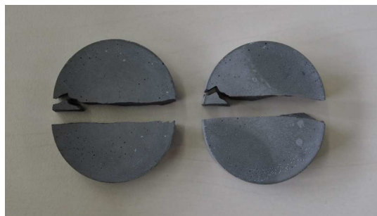
Figure 5.27.: Fractured Brazilian specimens with higher impact velocity.
