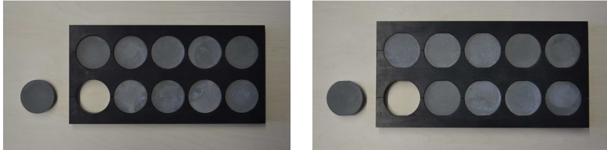
Figure 3.9.: The fabricated circular (left) and flat end (right) Brazilian specimens.
