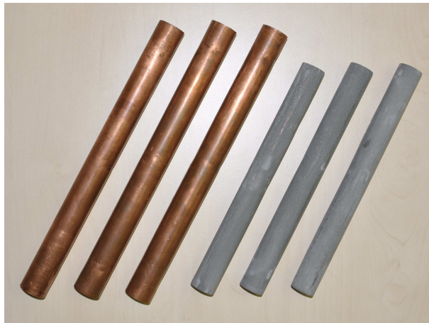
Figure 3.8.: Hollow copper tubes and prepared cylindrical UHPC specimens.
