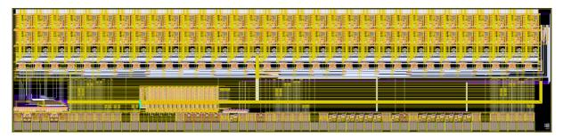
Figure 8.42 Layout of the complete chip 'Ramses 3' (6600  $\mu m \times 1515 \mu m$ )
