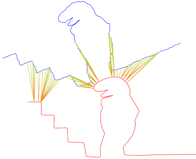
Figure A.2.1: Example of the brute-force ICP correspondences search (closest points) between the model curve (red) and the noisy input curve (blue). Note that here the correspondence set is trimmed using a maximum distance threshold.
