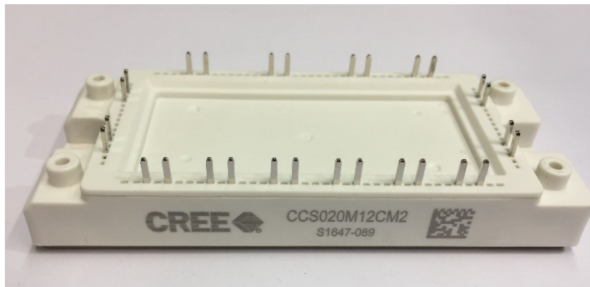
Figure 2-9 CCS020M12CM2 SiC MOSFET Cree module
