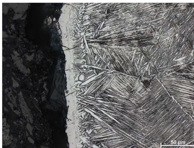
Figure 42. Microstructure of a cast Ti67 sample in \text{Al}_2\text{O}_3 based investment.
