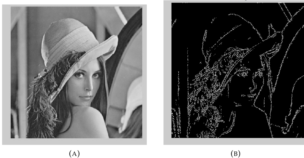
FIGURE 5.35: The Sobel edge detector. The left image is the original image, while the right one is the output after applying the Sobel filter, Source: [155].
