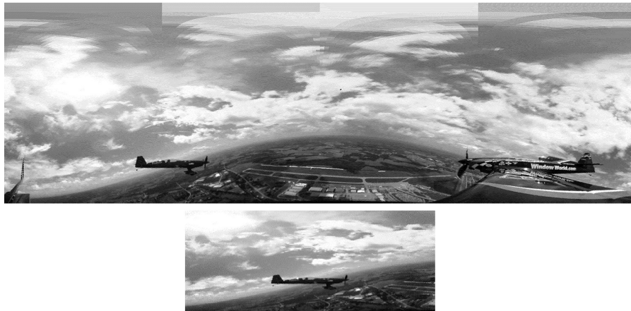
Figure 3.30: TLD searches the whole image to find the object of interest. This image shows rectified frame from the "Rob" video (top image). Limited searching area in MTLD is shown (bottom image). The probability of the presence of the object of interest in this region of interest (RoI) is higher than the rest of the image.
