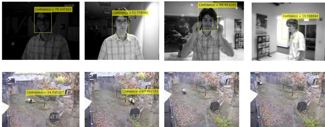
Figure 2.1: Challenges in two videos: First line (David) and second line (Panda) show illumination change, out-of-plane rotation, appearance change and background clutter changes, occlusion, articular objects, illumination change, and out-of-plane rotation. Some of the challenges are shown in Figure 2.1.
