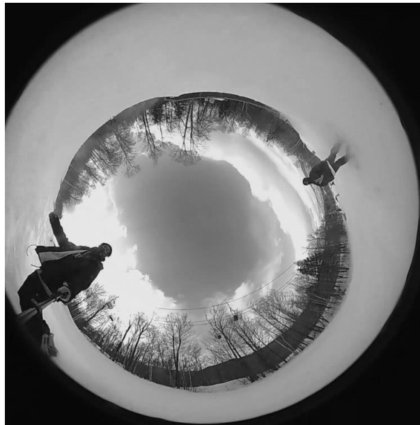
Figure 3.7: When YOLO is applied directly to the polar image, it cannot detect any object due to the object orientation.
