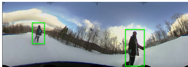
Figure 3.8: After image rectification, YOLO is able to state the correct position and size of the objects.
