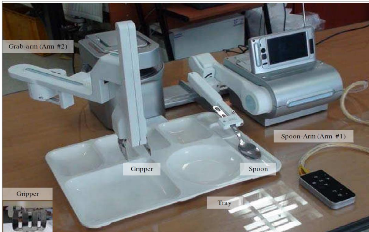
Figure 7: Assistive robot for self-feeding. Spoon arm (arm #1) uses a spoon to transfer the food from a container to a user's mouth. Grab arm (arm #2) picks up the food from a container and then loads it onto the spoon of arm #1 [20]
