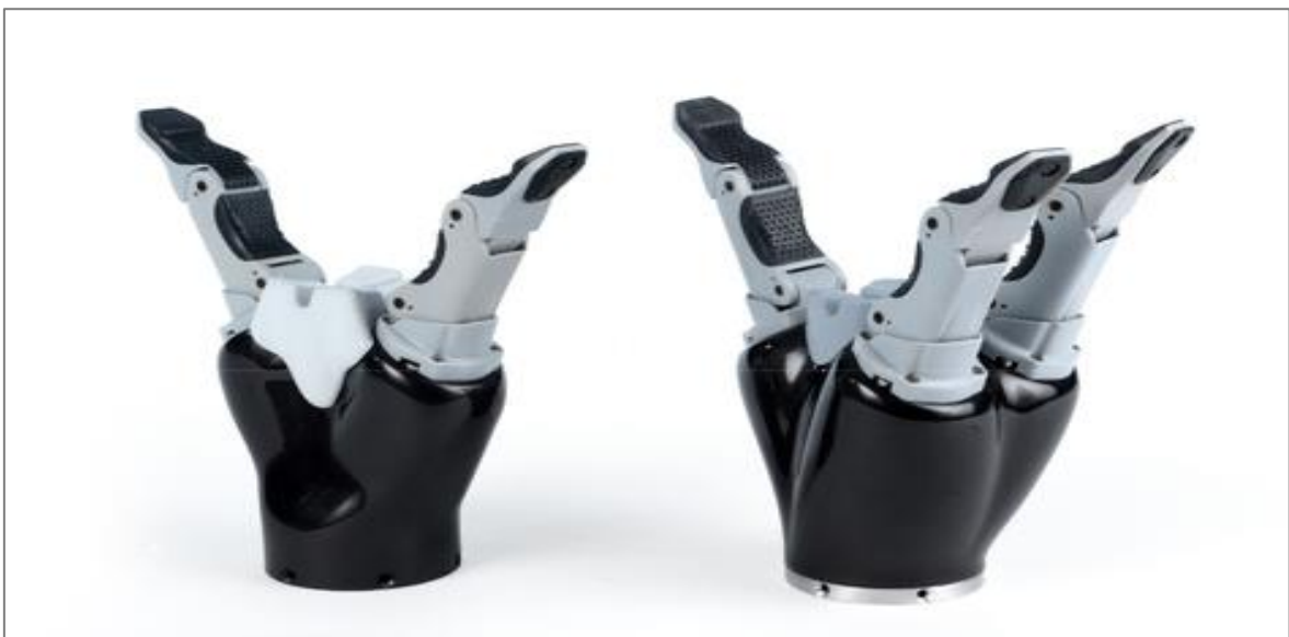
Figure 33: Gripper for JACO arm (two fingers, three fingers).[28]
