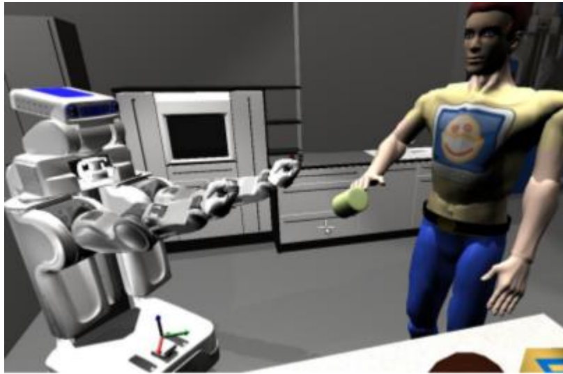
Figure 14: Simulation of a human model with an assistive mobile robot in MORSE [40].
