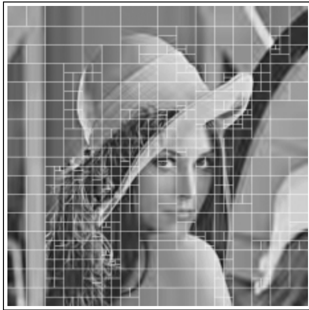
Figure 3.3: Bintree partitioning of the image Lenna.
