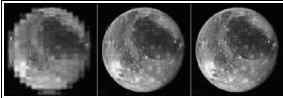
Figure 5.9: Progressive decoding of a WFA in wavelet mode.
