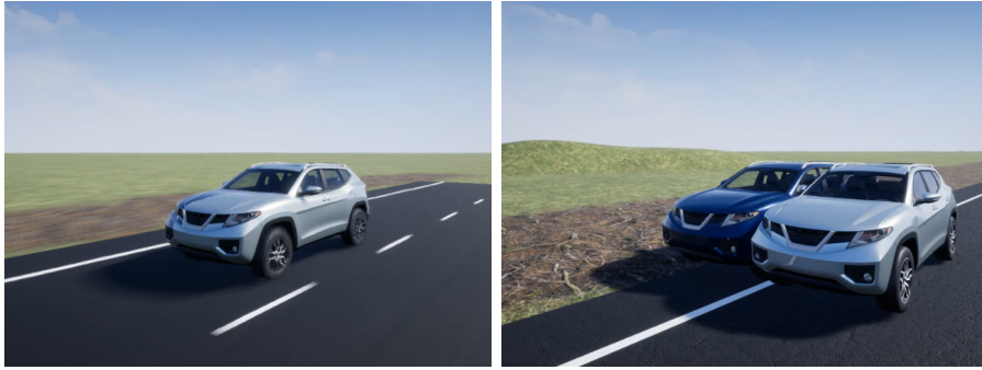
Figure 2.8.: 3D-visualization using Matlab/Simulink’s Vehicle Dynamics Blockset. Left: Two overlaid vehicles at the start of the emergency stop maneuver. Right: After 20s, the blue vehicle possessing a more accurate inertial sensor comes to a halt on the road shoulder, while the silver vehicle stops halfway on the road due to the worse performance parameters of its inertial sensor.
