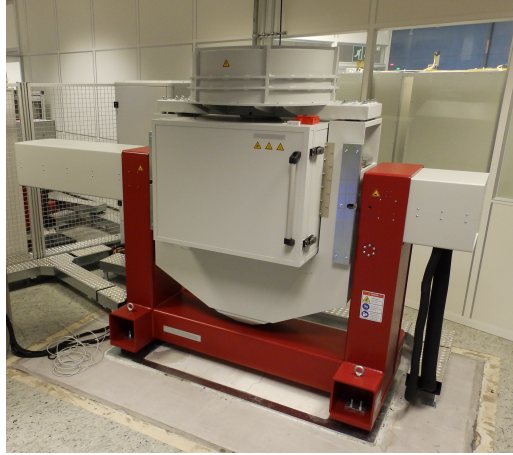
Figure A.13.: An ultra-high precision rotation chamber was used to analyze scale-factor instability effects by continuously rotating the sensors at a constant angular rate for extended durations on the order of 24 h and longer.
