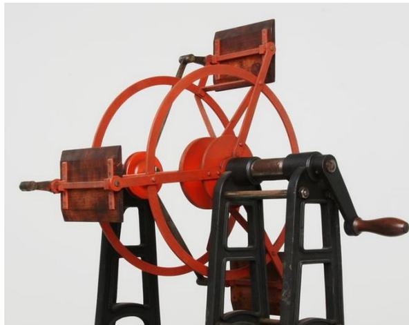
Abbildung 4-5: Modell des Buchanan's Feathering Paddle Wheel (Rudder, 2010)
