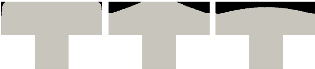
Figure 4.7.: The cavitation zone in the T-pipe segment for different viscosity factors: left to right \mu = 1 , \mu = 0.1 and \mu = 0.01 .
