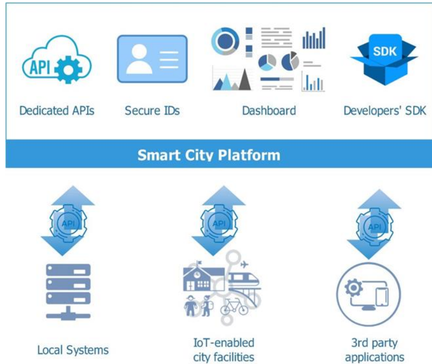
Figure 20.1 A generic SC platform architecture
