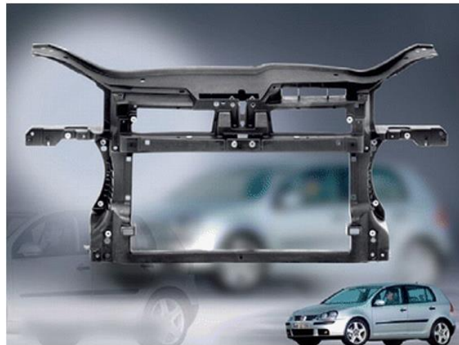
Figure 2-3 Typical LFT automotive component (a) [17]; Front end carrier for a VW Golf V (b) [15]
