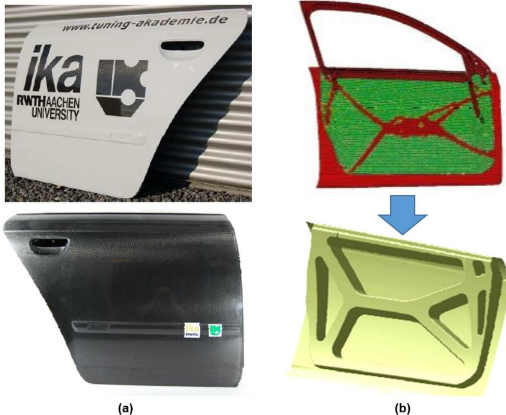
Figure 2-42 Multi-material door concept (a) and full CFRP door concept (b) from IKA [99]
