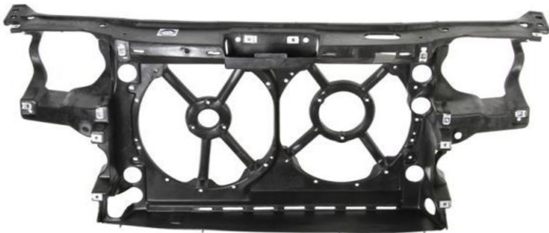
Figure 2-7 GMT front end carrier of the VW Golf 3 [39]
