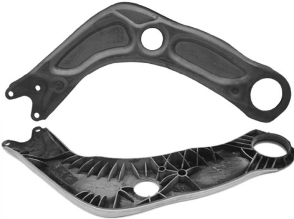
Figure 2-17 Front axle control arm made of “hybrid forming” [57; 62]
