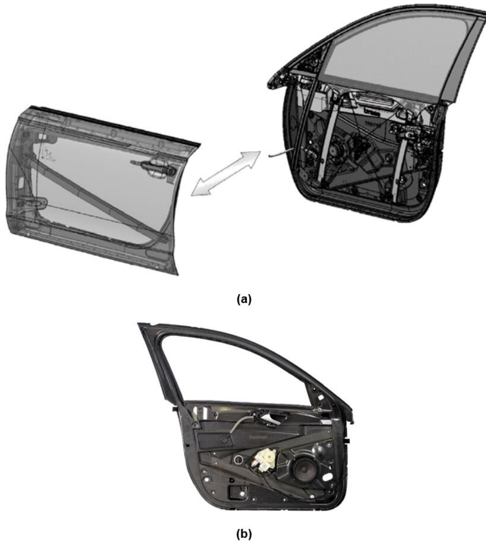
Figure 2-43 The CFRP-Door system from Brose Fahrzeugteile GmbH: assembled outer panel and inner panel (a); prototype (b) [100]
