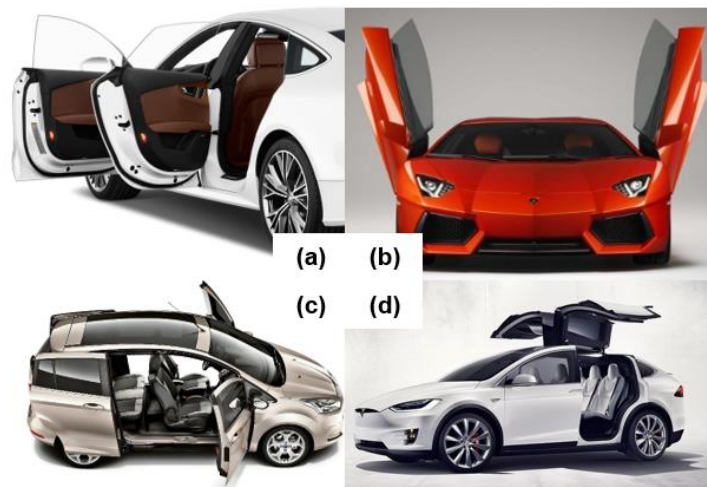
Figure 2-29 Typical appearances of vehicle doors. (a) regular turning door [79]; (b) scissor door [80]; (c) sliding door [81]; (d) falcon door [82].
