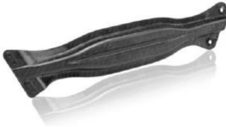
Figure 2-10 Door side impact beam from project “Spriform” [46]
