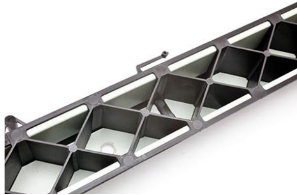
Figure 2-23 Erlanger Träger: steel sheet with PA6-GF ribs joined by a bonding agent [72; 73]
