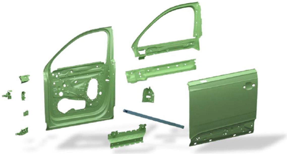
Figure 2-38 The Audi Q7 aluminum door (2015): Green components are made of aluminum sheets; blue components are made of aluminum extrusion profiles [96]
