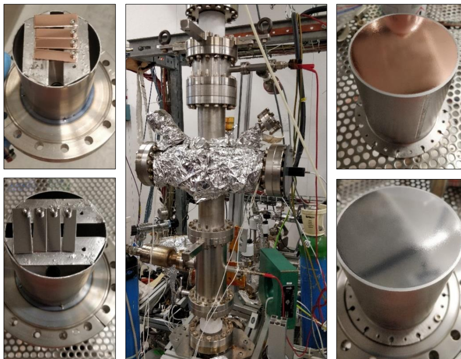
Figure 8-3: QPR deposition system used at CERN. Witness samples before (top) and after (bot) coating displayed on the left and the QPR sample before (top) and after (bot) coating displayed on the right.
