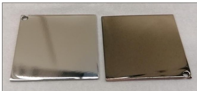
Figure 7-13: Image of NbN film deposited at low pressure (left) and high-pressure (right), displaying the change in colour experienced with an increase in deposition pressure.
