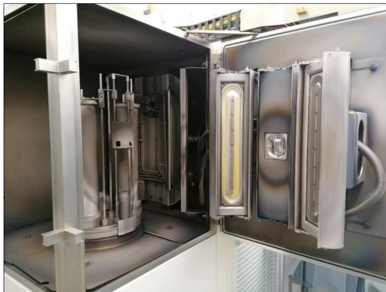
Figure 6-1: CemeCon CC800 industrial coating machine. Two of the doors have been opened to better visualise the deposition chamber.
