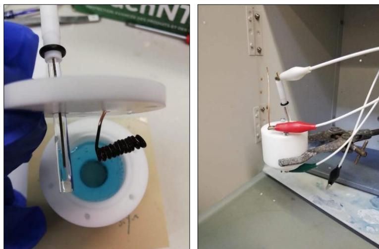
Figure 5-12: Images of the three-electrode cell used to perform the electrodynamic sweep of the anode-cathode-electrolyte combination. The anode is placed at the base of the cell, with a small section exposed to the electrolyte. The length of wire employed as the cathode was calculated based on the surface area ratio between the anode and cathode for sample creation.
