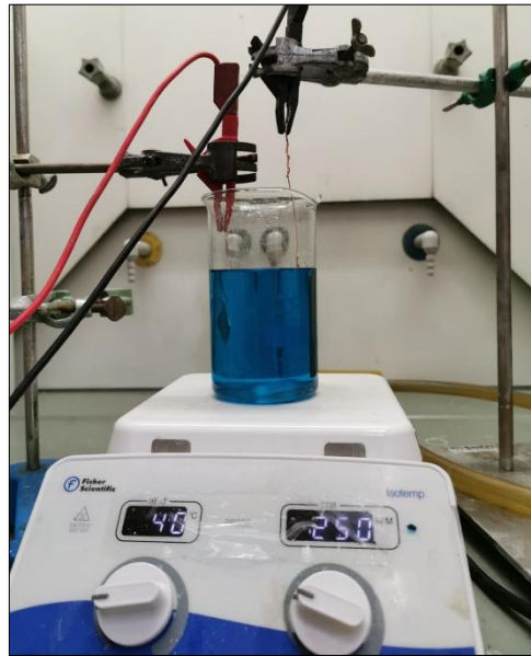
Figure 5-10: Image of the electropolishing setup used for sample preparation. The anode is connected to the red wire while the cathode is connected to the black wire.
