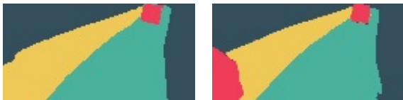
Figure 9: Two different predictions from the image in figure 8: The image on the right is a segmented output of a network trained only on real world data. On the left is the output of a network trained with synthetic and real data. This example demonstrated how synthetic data improve the classification of the under-represented class 'obstacle'.
