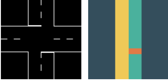
Figure 2: An image with its annotation representing an intersection chunk. The pixels of the image are assigned to a semantic class by their color (class 'left lane': yellow, class 'right lane': green, class 'obstacle': red, class 'intersection': orange).
