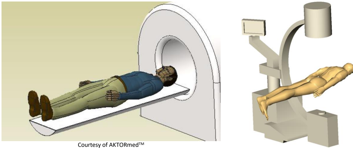
Figure 5-49. Patient positioning during modalities acquisition for spine surgery. CT-scan on the left, X-ray on the right
