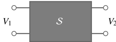
Figure 1.2: Representation of a system, S , as a two-port network with port voltages V_1 and V_2
