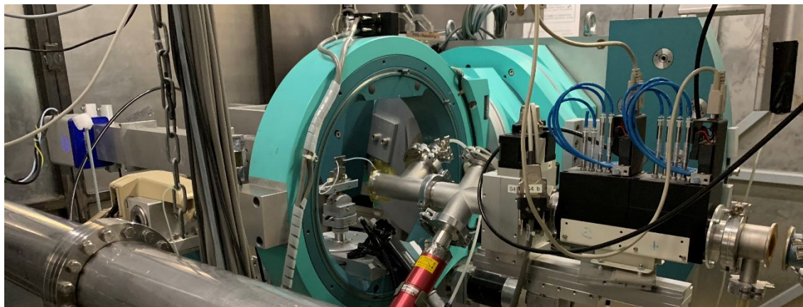
Figure 3.5 The SAXS experimental setup at BL9.
