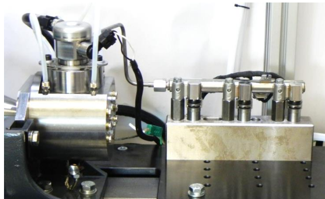
Figure 50: Build up gasoline high pressure pump test build up with mounted Kefico 250 bar GDI pump
