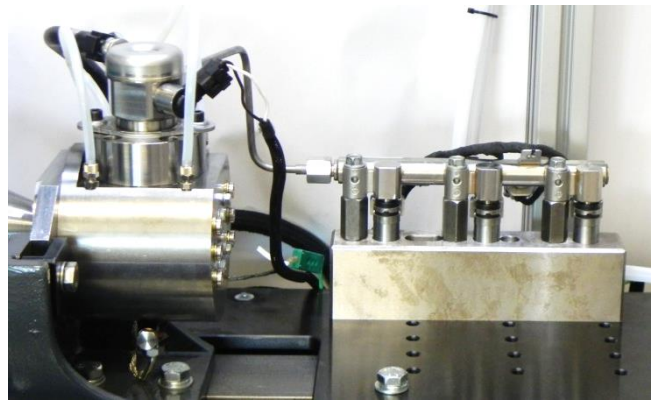
Figure 35: Build up gasoline high pressure pump test build up
