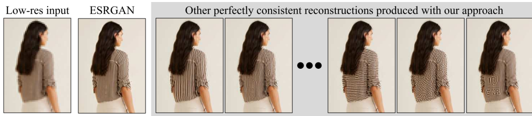
Figure 3.3: This figure is taken from Bahat et al. [16] and shows on the left a low-resolution image, and multiple corresponding high-resolution images, resulting from the exposable super-resolution approach in [16], where all high-resolution images are consistent with the low-resolution image.
