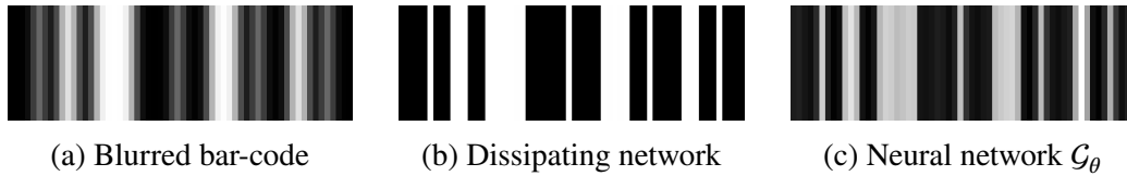
Figure 7.5: Deblurring results for the blurred input bar-code using a Gaussian filter with radius 1.0 (a), by running descent on an energy dissipating network (b), satisfying (7.38), and by applying a trained neural network (c).
