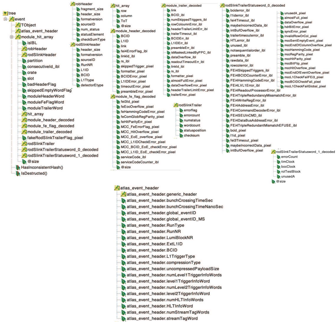
Figure 4.9: Structure of the output in ROOT TTree format. A class structure is defined to store the decoded information, which is saved as a tuple using the ROOT::TTree library. Event metadata is stored for each event in atlas_event_header . The module_hit_array is an array structure containing information for each ROD fragment. Hits processed by a single ROD are stored within hit_array , another array structure. The hit_array includes detailed hit information for every hit in the pixel detector.
