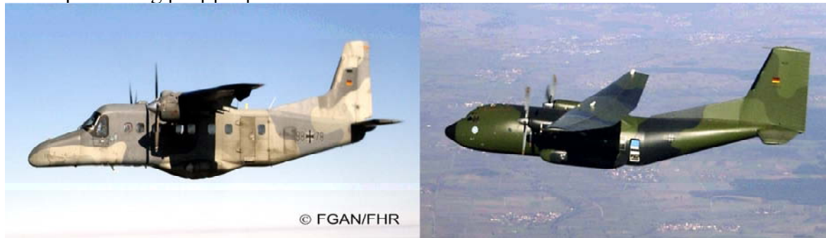
Figure 8.9 FGAN's transmitter on Do-228 (left) and receiver on Transall-C160 (right)
