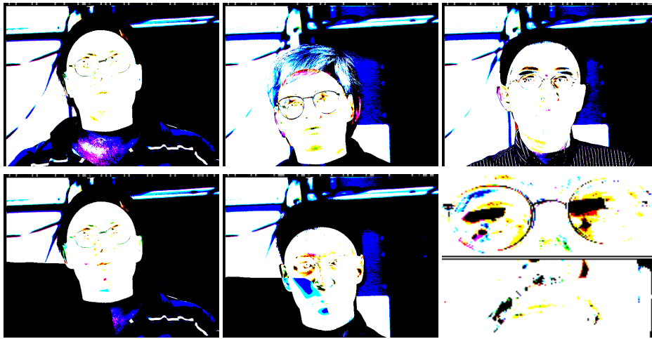
Figure 8.9: Average of differences per color channel: Here the differences have been computed separately for each color channel and the combined results are presented. The shown colors indicate in which channel an occlusion has been detected. white: nowhere, black: in every color channel, cyan: red channel only, magenta: green channel only, yellow: blue channel only, blue: red and green channel, green: red and blue channel, red: green and blue channel
