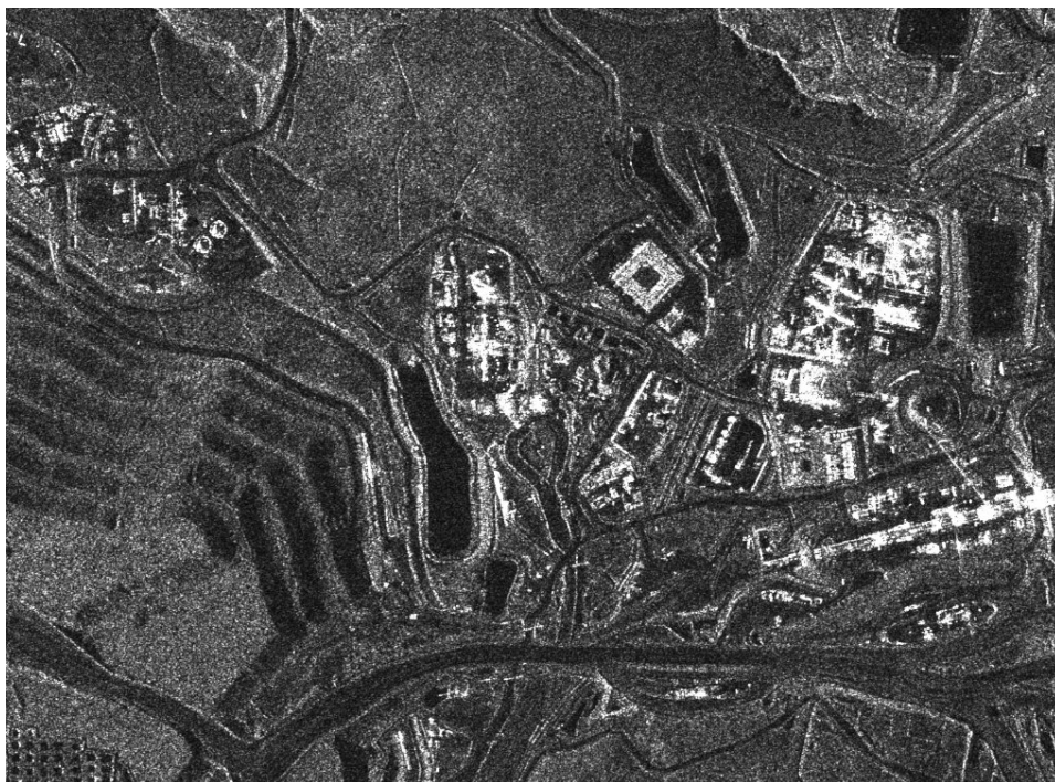
Figure 2.2: The SAR amplitude image from Fig. 2.1. To produce this image, the lowest 10% of the amplitude range was linearly mapped to gray levels. The highest 90% of the amplitude range was clipped to white, and all details in this range are lost.
