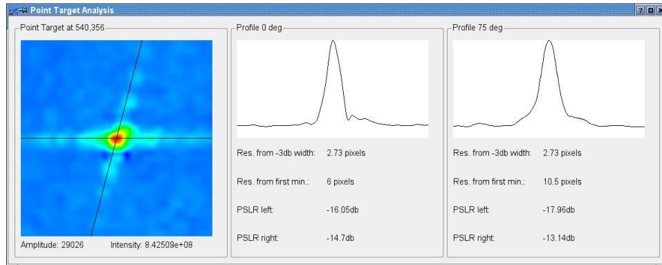
Figure 2.13: Example of a point target response analysis window, displayed on user demand.
