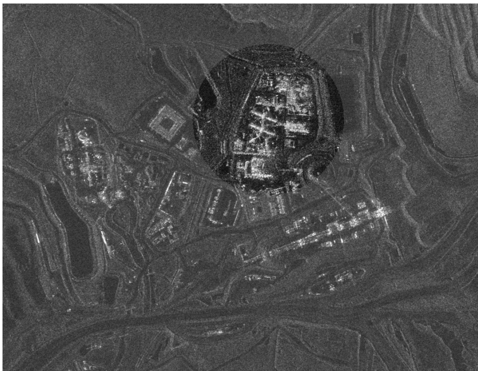
Figure 2.4: Global and local dynamic range reduction methods applied simultaneously to a SAR image using a lens.
