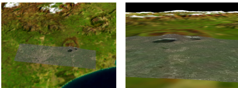
Figure 1.17: The area around Rome, Italy, in a combined view of two DEM data sets, a false color image, and a SAR amplitude image.
