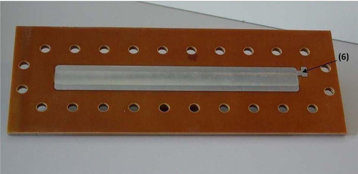
Figure 4-2: The design of the cathode (13 μm thick aluminum foil) for multi-channel ionization chamber construction.
