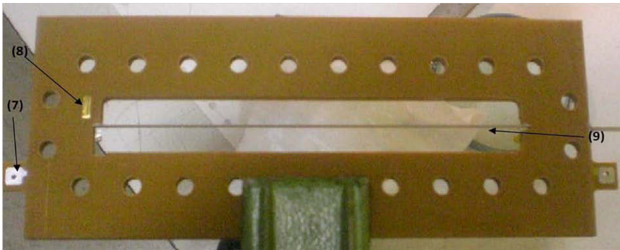
Figure 4-3: High voltage connection for the multi-ionization chamber. High voltage contacts (7), feed through contact for the cathode (8) and Central electrode (9).
