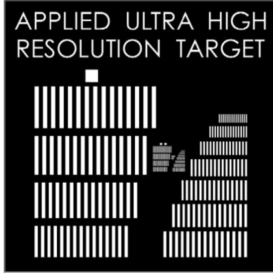
Figure 5.12: Ultra high resolution target for use in the lateral focal-interval calibration. The black area represents the glass plate, whereas the white area depicts the chrome layer of periodic patterns.
