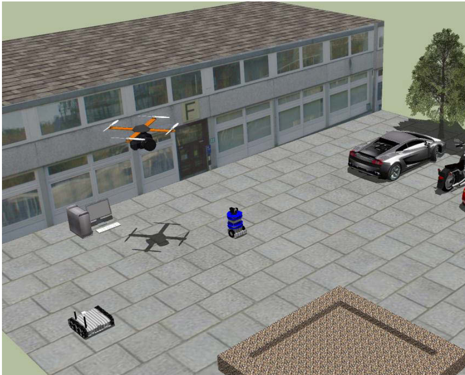
Figure 5.1 Heterogeneous mobile robots cooperation for map building in a partially structured environment
