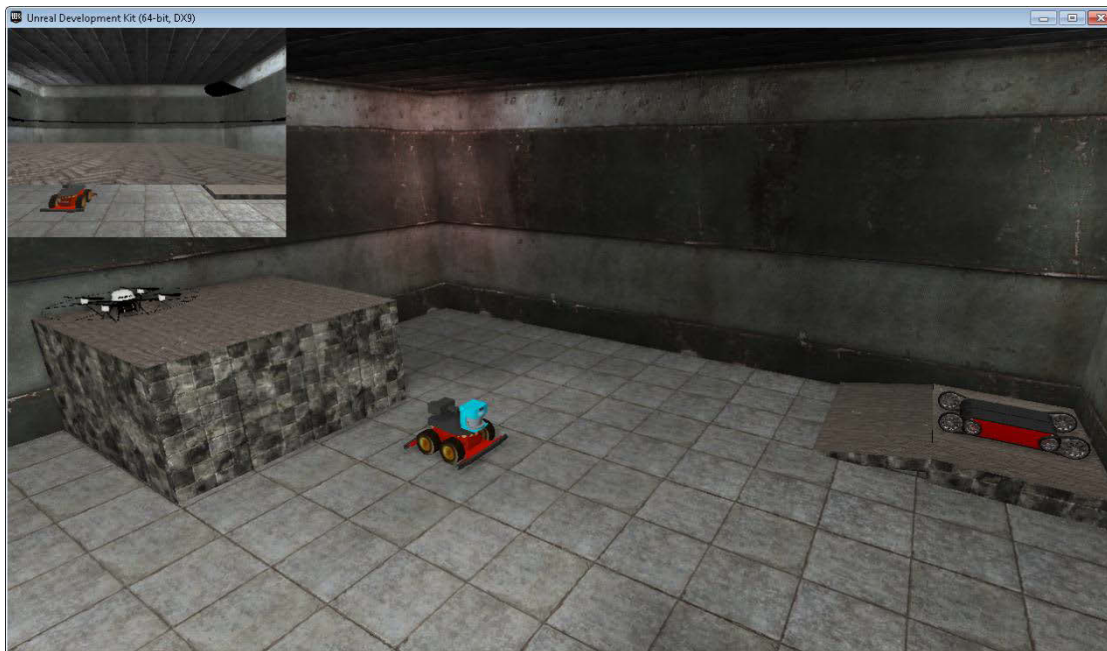
Figure 1.4 Simulation of aerial and ground robot in a virtual environment based on Unreal Tournament game engine
