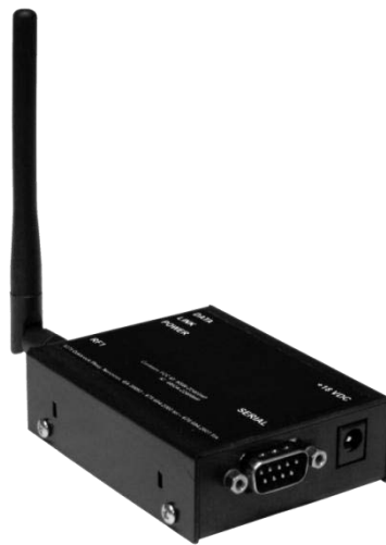
Figure 5.18 Agents Communication Modem based on IEEE 802.15.4
