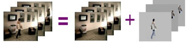
Fig.2. Image sequences can be formulated as a sum of background sequences and image sequences which only contains the moving human.
