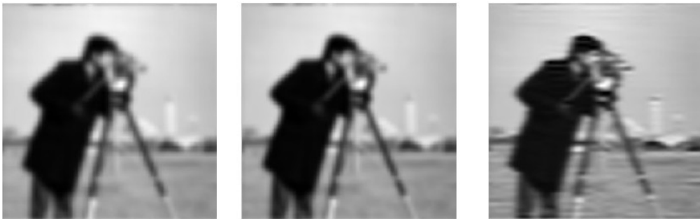
Figure 4. (a) SR result from Fig.3 (c) via ‘bilinear’ interpolation. (b) SR result from Fig.3 (c) via ‘bicubic’ interpolation. (c)SR result Fig.3 (c) via the proposed method.
