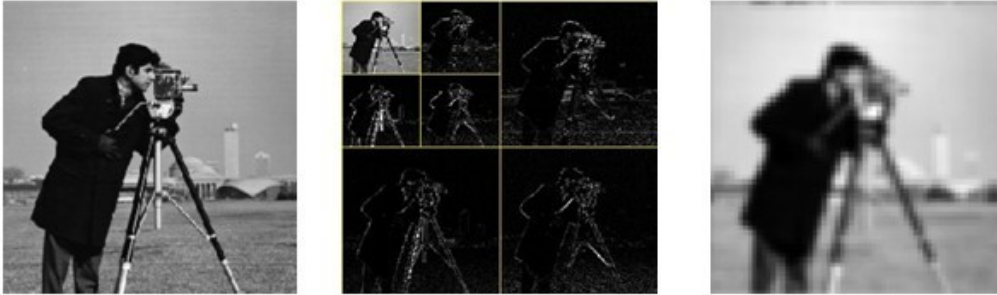
Figure 3. (a) The original HR image. (b) The corresponding wavelet transform with ‘haar’ at level 2. (c) The LR image after applying Gaussian low-pass filter and decimation operators.
